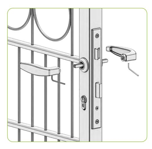
Insert the doorhandle pin through the lock and out through the other side. Slide the doorhandles on the pin on both sides and tighten them with the Allen key provided.
