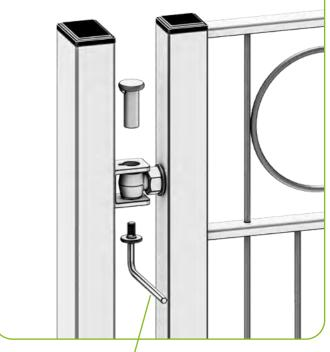
Make sure that the hole of the hinge plates on the post and the hole of the eye bolt are aligned and insert the hinge bolt through them and turn the bolt until it is stuck in the recess. Finally, tighten the small bolt with an Allen key. If the gate does not fit completely, you can still adjust the eye bolt.
