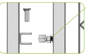
If you have too little or too much space between the posts than you had in mind, you can adjust the position of the eyebolt in the hinge plate by adjusting the position of the nuts on the eyebolt.
