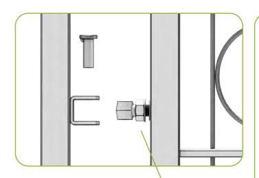
Tighten the nut on the eyebolt well so that the gate leaf is firmly attached to the eyebolt. Then hang the gate leaf in position.
